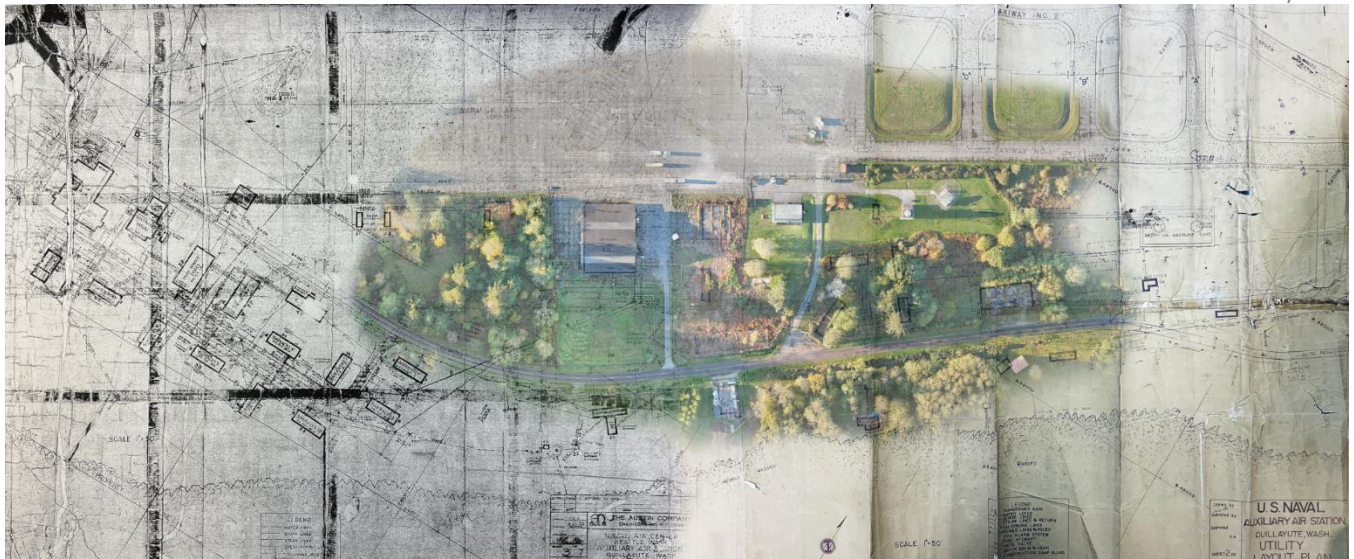
Figure 9: transparent overlay of apron orthographic imagery with historic drawings
